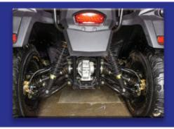
Conquer rough terrains and tough jobs with the ability to switch drives systems with the dual a-arm independent rear suspension. These shocks have five adjustable pre-loaded settings and variable spring rate for optimal performance.
